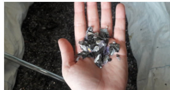
Phenix Recycling, example of chipped plastics
