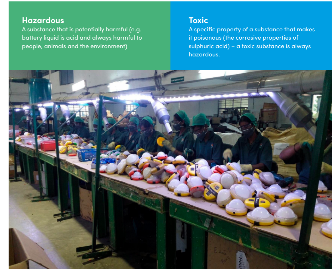
E- Parisaraa Private Limited. Dismantling of solar lights
