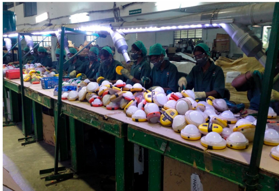
E- Parisaraa Private Limited. Dismantling of solar lights
