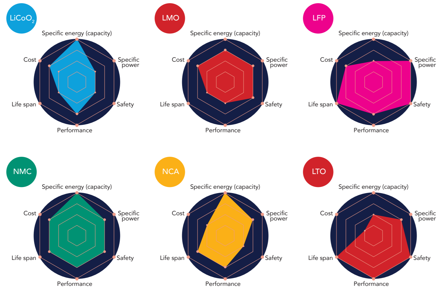
Figure 2 Comparison of characteristics of common lithium-ion types 6 .
